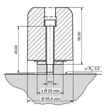
FAG SmartCheck installed with sensor mounting plate
