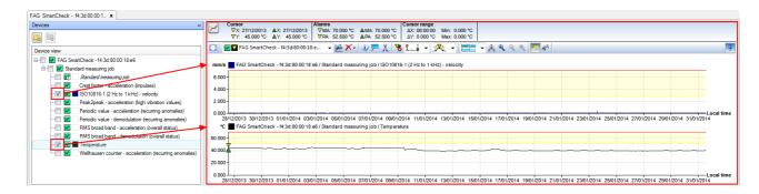
With each additional open trend, the Time Signal and Spectrum Viewer are also adjusted: If the **Load most recent data set** option has been activated, the last available time signal will be loaded in the Time Signal and Spectrum Viewer for each loaded trend.
