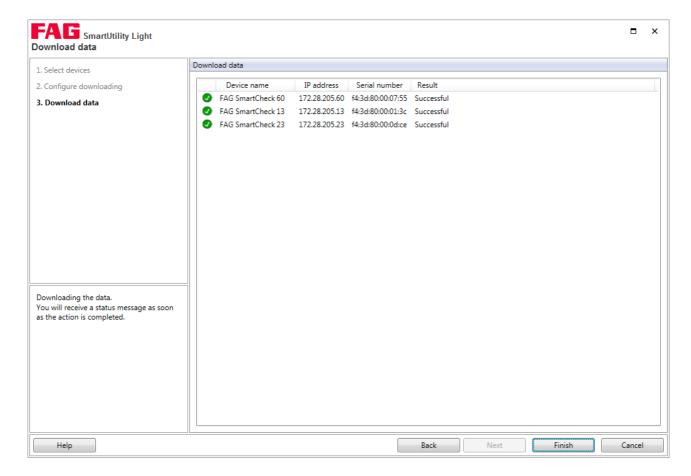
The downloaded measurement data can be found in the Default directory for data in the SmartUtility Light software or in the directory that you specified in **Step 2**. An individual subdirectory is created for each SmartCheck device. The name of this subdirectory is the serial number of the device.
