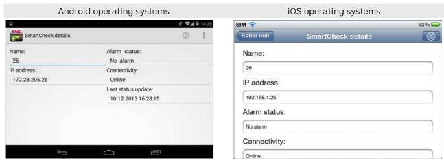
The SmartCheck device details are displayed together with the following information: name, IP address, alarm status, connectivity and last alarm status update.
